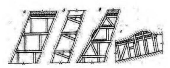
$\checkmark$  Structure reinforced with a pillar reinforcement, in the mining of ore located close to the vertical  $(a, \delta, B)$  and when the ore body is slightly inclined (g).
