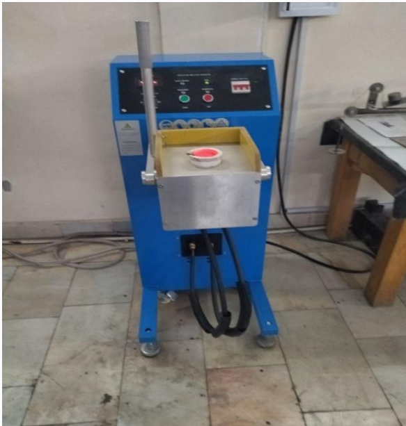
1-rasm. Induksion eritish pechi (Model: BF-TB2)
